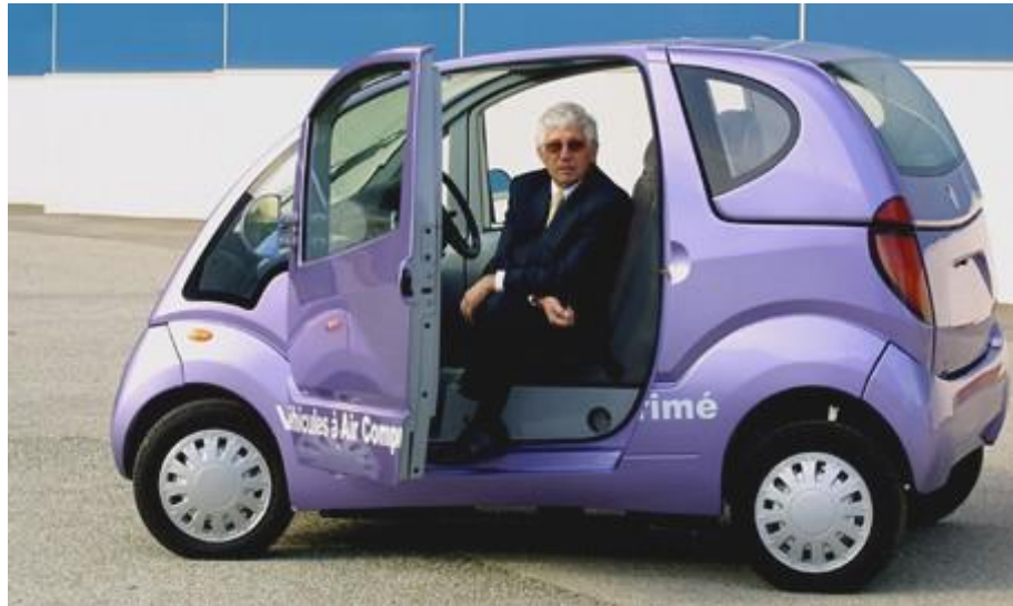
The "MiniCAT". It runs of Compressed Air
