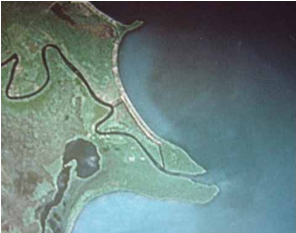
This satellite photo shows the area of development on a small bay near the Sittee River mouth. Note the lighter color of shallow water and the bay, both of which would increase a storm surge.
