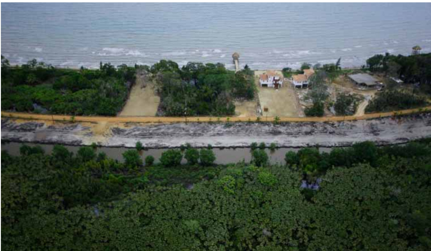
This aerial view shows homes built along the coast cleared of protective mangroves and the canal dug behind. A storm surge could wash across beach into canal and possibly divert the river.
